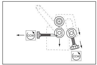
Figure 12. Slip roll preparation.
